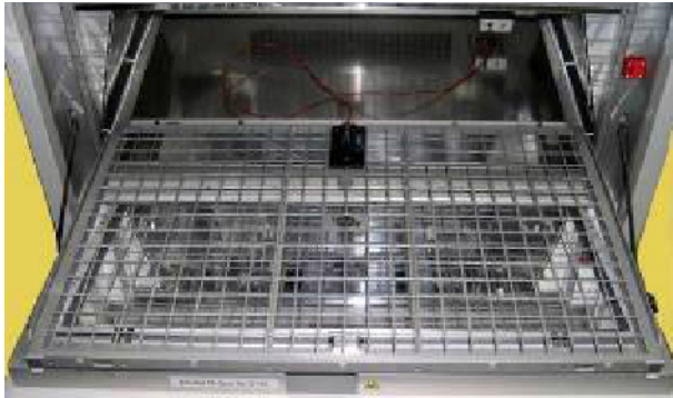
Figure 5.b: Open Mesh Sample Tray - Install Under Horizontal Specimen Tray Insert
