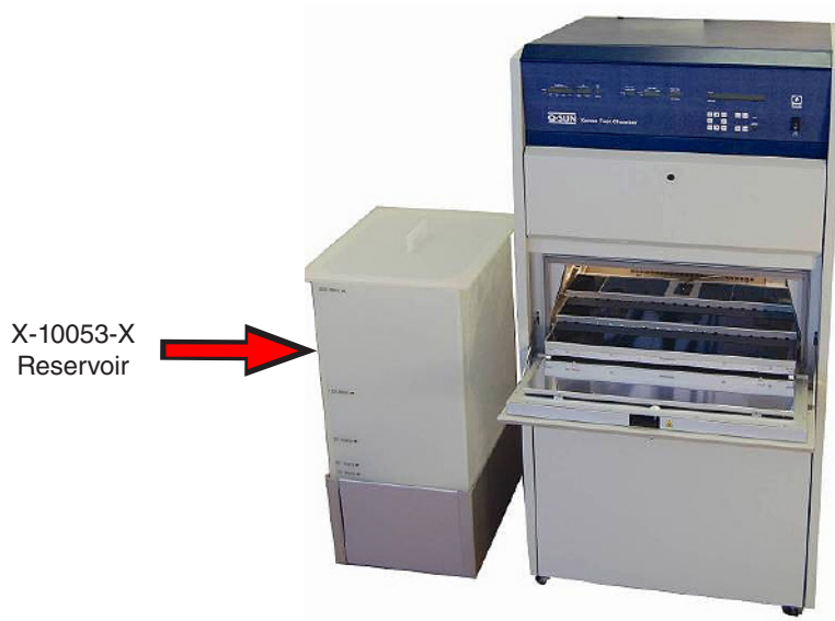
Figure 7.c: Reservoir Dual Spray System
