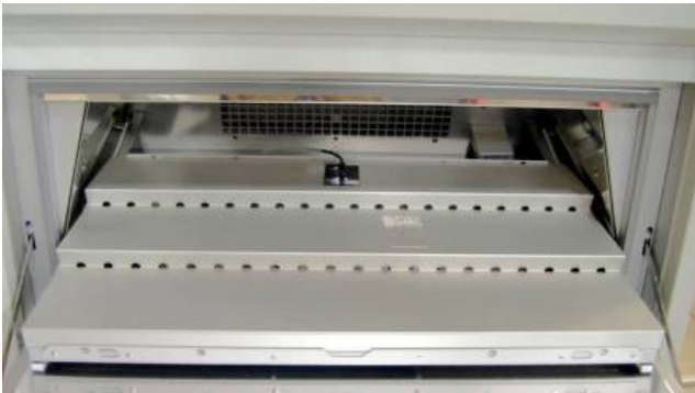
Figure 5.a: Horizontal Specimen Tray Insert - Install on Top of Open Mesh Tray so Liquid Will Pool and Not Run Off the Specimens
