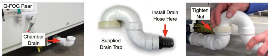
Figure 5.8a: Drain trap installation.
