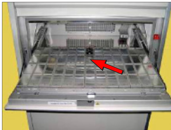
Figure 11.4ab: Reference material position on specimen tray (with panel holders).
