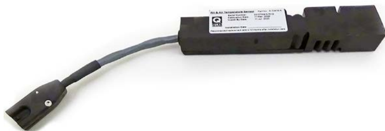
Figure 8.2b: RH (and chamber air temperature) sensor.
