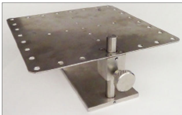
Figure 14.5a: 3D Specimen Stand - All 5 stands included in the kit must be placed in the chamber.
