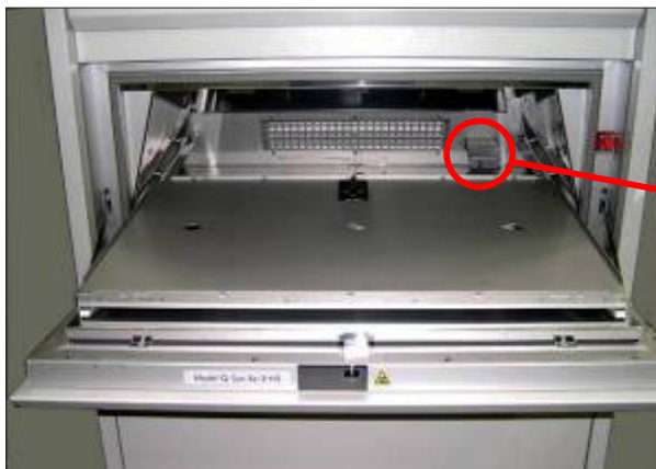
Figure 12.4a: RH/Chamber Air Temperature sensor location.
