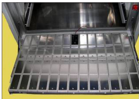
Figure 11.4i: Panel holder kit (Part Number X-10114-K) with (26) panel holders holding (51) 50×100 mm specimens and the black panel.
