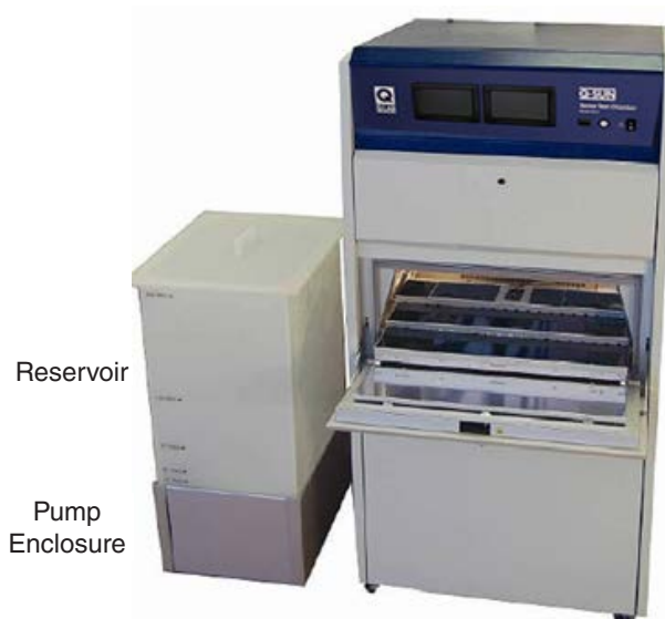
Figure 2.3: Dual Spray reservoir and pump system enclosure.
