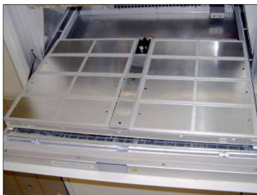
Figure 11.4k: Panel holder kit (Part Number X-10261-K) with (8) panel holders holding (16) 100x150 mm specimens and (2) 50x100 mm panel holders.
