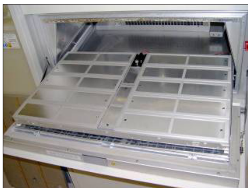
Figure 11.4j: Panel holder kit (Part Number X-10260-K) with (10) panel holders holding (20) 75x150 mm specimens and (2) 50x100 mm panel holders.
