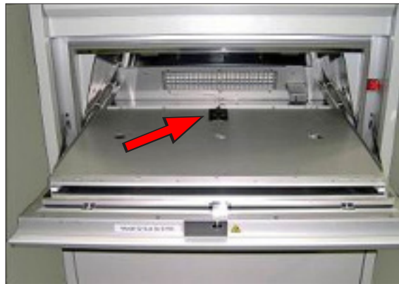
Figure 7.1f: Proper location of the panel temperature sensor.
