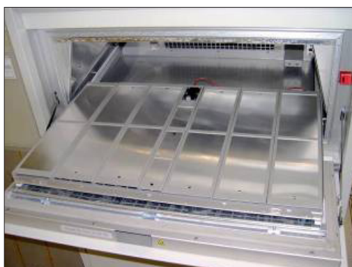
Figure 11.4l: Panel holder kit (Part Number X-10262-K) with (6) panel holders holding (12) 100x200 mm specimens and (2) 50x100 mm panel holders.
