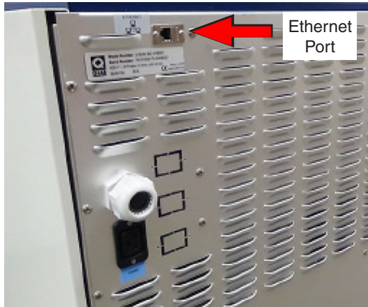
Figure 13.1a: Ethernet port located at the top left corner of the tester back panel.
