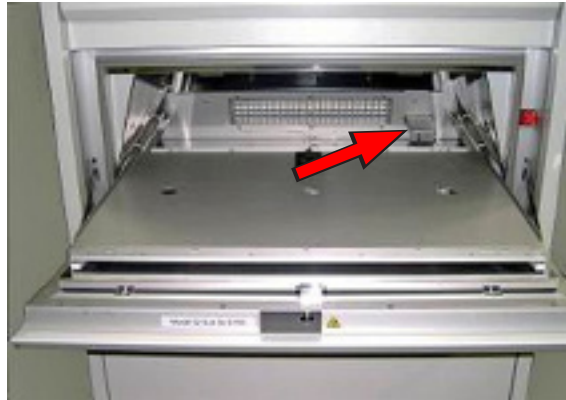
Figure 7.2a: Chamber air temperature sensor location.
