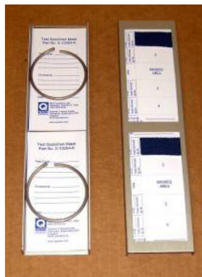
Figure 11.4y: Textile mask mounted in panel holder with one section of the mask removed.
