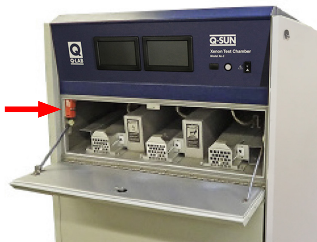
Figure 2.1d: Lamp Door Interlock Switch Location
