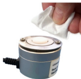
Figure 12.1e: Clean the sensor face with 99% isopropyl alcohol and a soft cloth.
