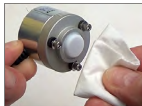
Figure 13.1e: Clean the sensor face with alcohol and a soft cloth.
