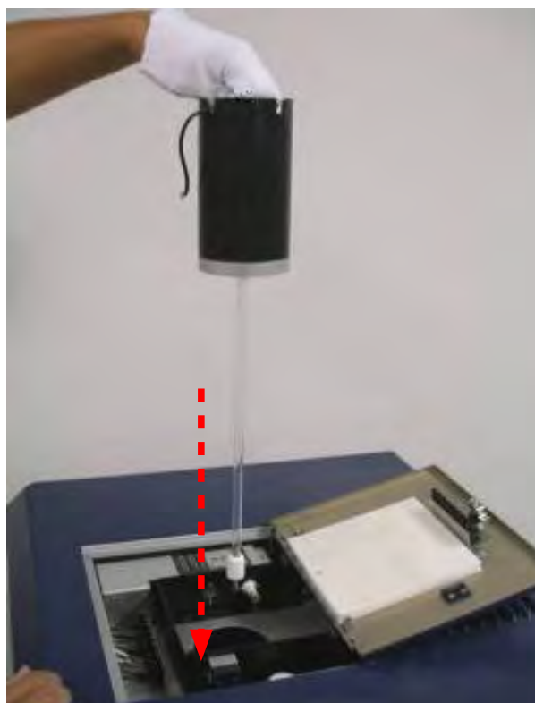
Figure 16.1h: Carefully lower lamp into the tester.
