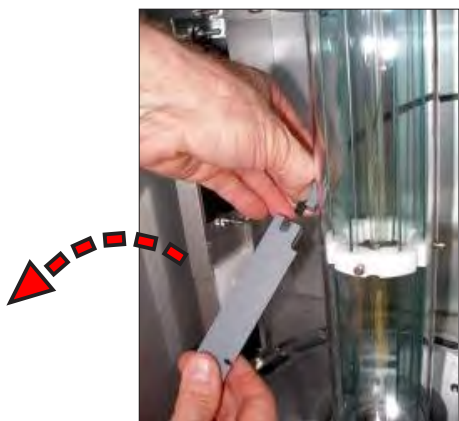
Figure 13.4c: Push the release lever on the connector to disconnect the sensor from the cable. Discard the old sensor.
