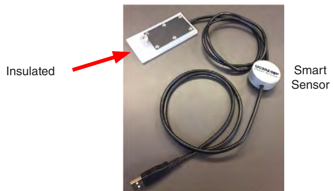
Figure 13.2b: UC202/IBP Temperature Smart Sensor with Insulated Black Panel (Black Standard)
