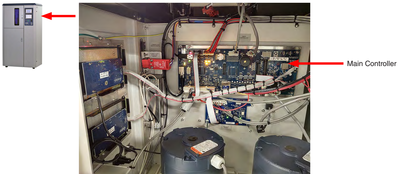
Figure 7.5b: Right side door open showing main controller.
