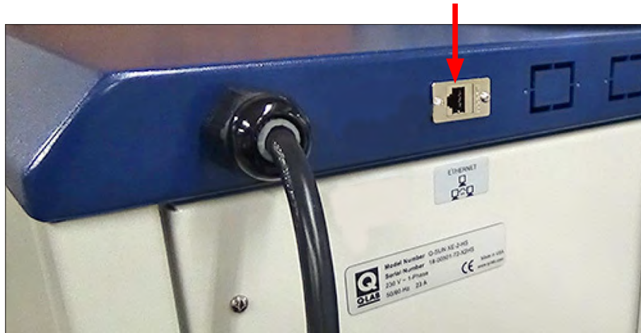
Figure 14.1: Ethernet port located at the top left corner at the rear of the tester.
