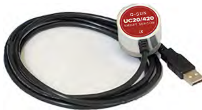
Figure 13.1b: UC20/420 Smart Sensor (Red Label)
