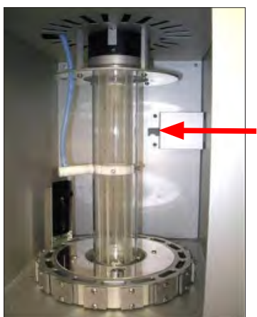
Figure 13.4a: RH/Chamber Air Temperature Sensor at the right rear of the test chamber.
