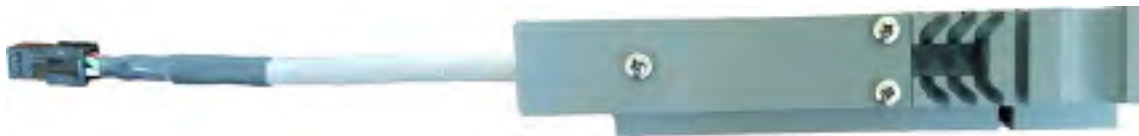
Figure 8.3b: Chamber air temperature (and relative humidity) sensor.
