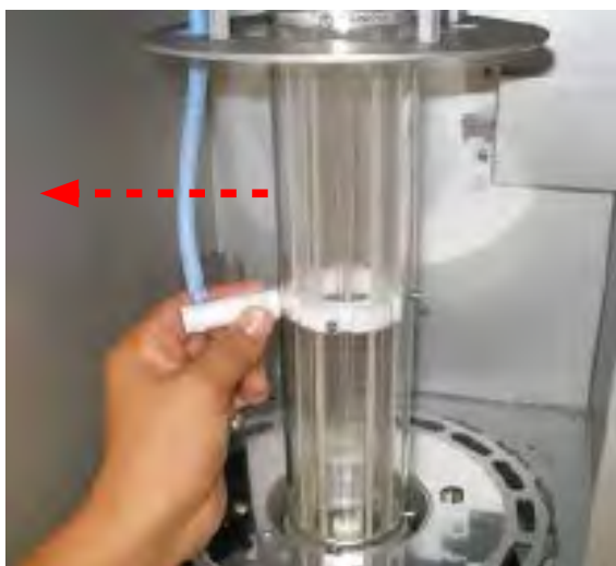
Figure 16.2.1a: Remove trigger wire from lantern.
