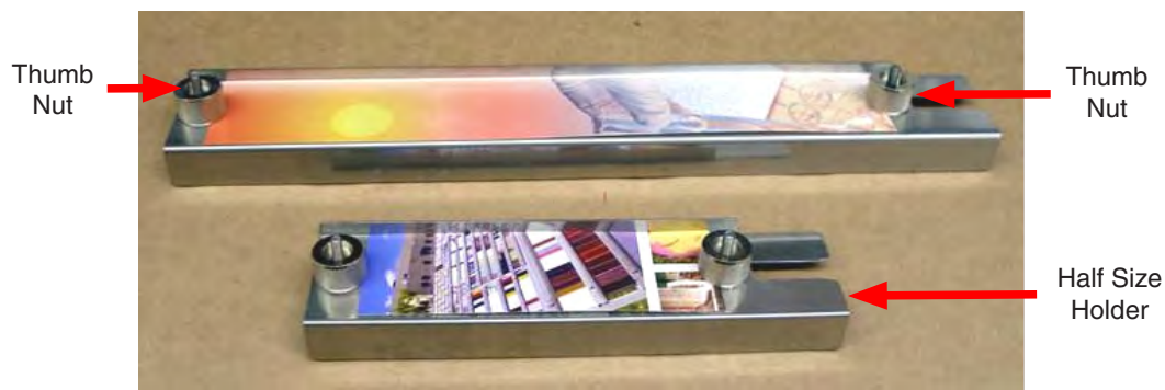
Figure 12.3g: Solid back specimen holder.
